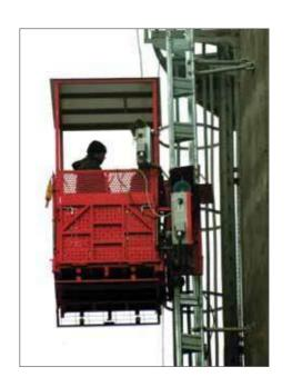
IZA 750 is an interior and exterior material hoist with high performance which you can use in constructions for the works of surface coating, paint, sheathing and for carrying construction materials to upper floors. Can be used in your intense construction works, material transporting and unloading and in places where tower crane can not reach. Easily replaceable.
